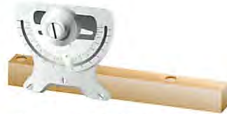
This is a picture of one type of clinometer, called an Abney hand level and clinometer. (Courtesy of Keuffel & Esser Co.)
